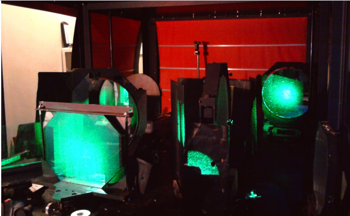
Equipment for (a) fabrication and (b) testing of VPH gratings at State Inst. Of Applied Optics (Kazan)
