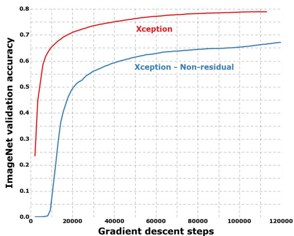
Figure 9. Training profile with and without residual connections.
