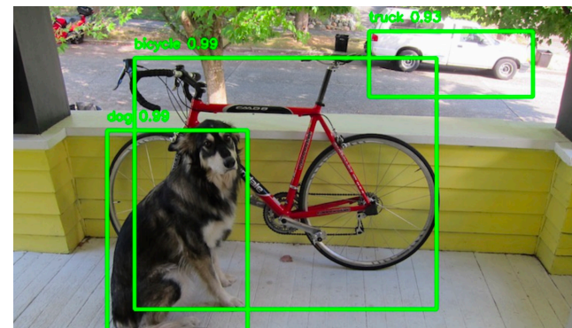
End of 2010s : Real time detection of more than 1000 image features using CNNs in 24 fps videos (Yolo v3).
